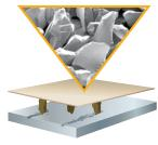
Conventional ceramic abrasive grain tends to "plow" through the metal, causing heat to build up in the workpiece and the abrasive — resulting in a slower cut and shorter disc life.
