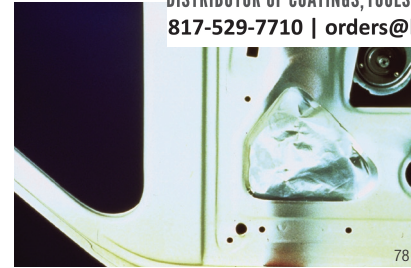
Applied over holes and cavities in the interior of a car or truck door panel, 3M™ Aluminum Foil Tape seals out moisture and dust.
