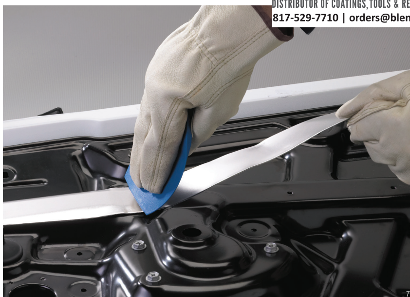
Applied with a 3M™ PA-1 Wiper to the inside of a car door, 3M™ Damping Foil 2552 effectively damps noise and vibration with as little as 10% surface coverage. Optimized acrylic on a dead soft aluminum constraining layer converts vibrational energy to negligible heat that readily dissipates.
