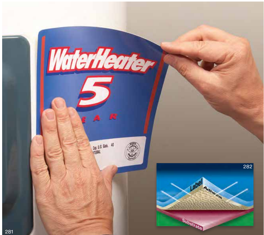
3M™ Performance Label Materials with Structured Adhesive – With unique microchannels throughout the structured adhesive, air flows freely from between the label adhesive and substrate. Hand-applied large labels go on smoothly and stay that way permanently without unsightly wrinkles and bubbles.
