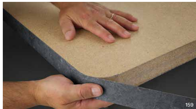
3M™ Hi-Strength 90 Spray Adhesive has a long reputation of holding strong in critical applications like this edge band that are postformable. Postforming is where the laminate is heated and bent as much as 360° around a radius.
